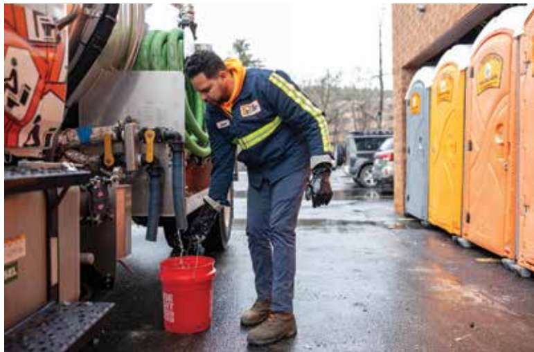
Ortega uses the convenient bucket fill on his truck to recharge restroom holding tanks following a pumping.
